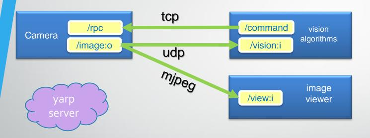
YARP server acts as a DNS, resolving yarp port names into system sockets
