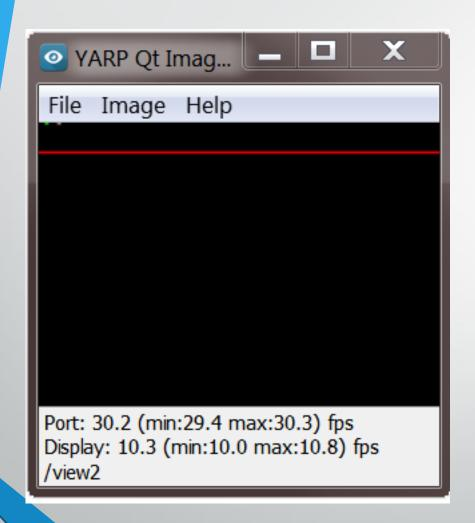
yarpview is a graphical interface for viewing images transmitted on the YARP network.
