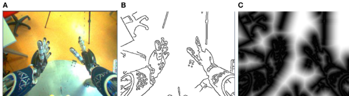
FIGURE 5 | Example of the computation of the edges and distance transform of the iCub hand in a real environment on the right camera. (A similar example can be shown for the left camera.) (A) is the input image, (B) shows the edges extraction using Canny, 1986, and (C) the distance transform using Borgefors, 1986.
