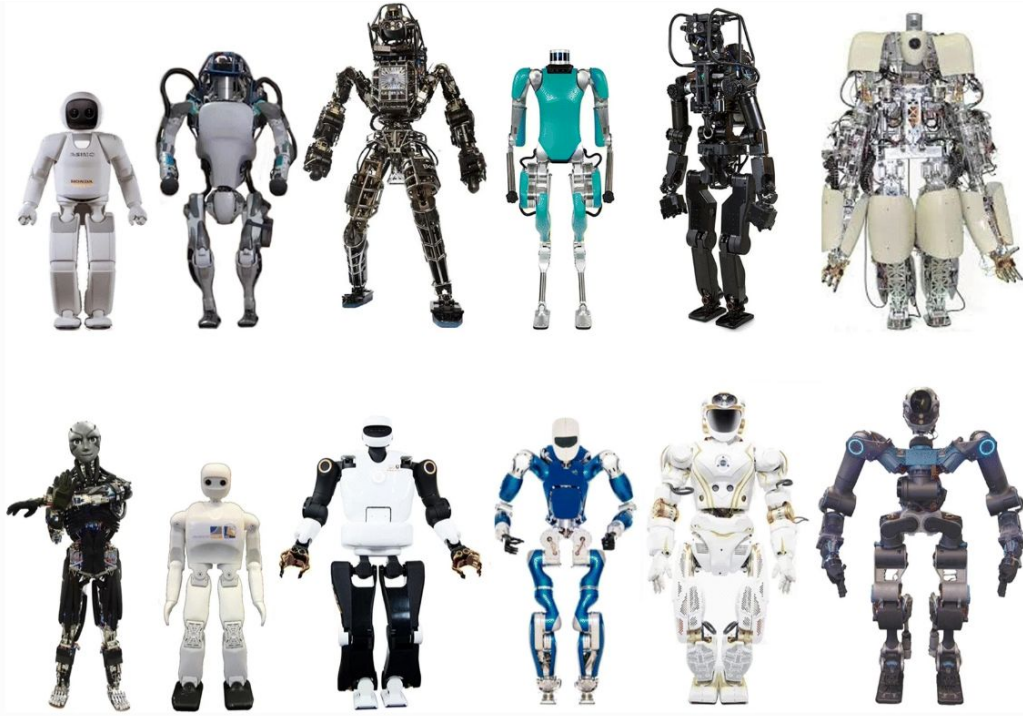
Most recently developed bipedal humanoid robots with a full humanoid body plan, from left to right, top to bottom: Asimo, Atlas, Atlas-Unplugged, Digit, HRP-3P, Hydra, Kengoro, NimbRo-OP2X, TALOS, Toro, Valkyrie, WALK-MAN
