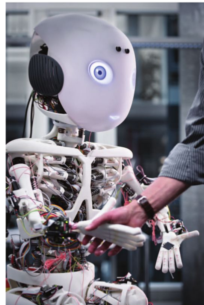
Figure 7. Roby, a human-like, musculoskeletal robot with 28 degrees of freedom and 48 motors, to be controlled by brain-inspired systems. (Photograph courtesy of Adrian Baer.)
