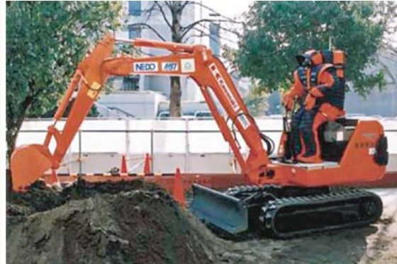
Fig. 56.1 The humanoid robot HRP-1S driving a backhoe (Courtesy of Kawasaki Heavy Industries, Tokyu Construction and AIST). The robot can be teleoperated by a human operator to control the backhoe remotely. The same robot could potentially interface with many different unmodified machines
