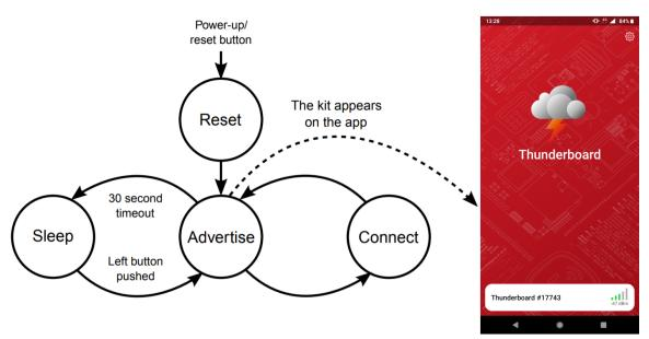
You can connect the device by tapping on the name of it in the Thunderboard app. After the connection is established, you will see the dashboard. There, you can select the categories of the different sensor types and the controls to see.
