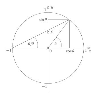
Figure 8.2: Cayley transform parameterization of two-dimensional rotations.
