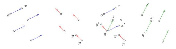
Figure 4.8: Free vector  $A_{(o,x)}$  is added to free vector  $A_{(p,y)}$  by translating (o, x) to (q, x') and (p, y) to (q, y'), adding bound vectors  $(q, z) = (q, x') \oplus (q, y')$  and setting  $A_{(o,x)} \boxplus A_{(p,y)} = A_{(q,z)}$
