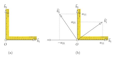
Figure 5.2: Rotation in two-dimensional space.
