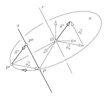
Figure 7.2: Axis *a* of motion is parallel to the axis of rotation *r* and intersects the perpendicular plane  $\sigma$  passing through the origin *O* at a point *P*, which is first rotated in  $\sigma$  away from *a* to *P'* and then returned back to *P''* on *a* by translation  $\vec{\sigma}'$ . Point *P* is determined by the component  $\vec{\sigma}'_{\sigma}$  of  $\vec{\sigma}'$ , which is in the plane  $\sigma$ .
