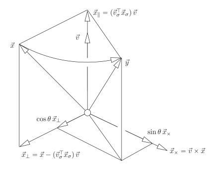
Figure 8.1: Vector  $\vec{y}$  is obtained by rotating vector  $\vec{x}$  by angle  $\theta$  around the rotation axis given by unit vector  $\vec{v}$ . Vector  $\vec{y}$  can be written as a linear combination of an orthogonal basis  $[\vec{x} - (\vec{v}_{\sigma}^{\top} \vec{x}_{\sigma}) \vec{v}, \vec{v} \times \vec{x}, (\vec{v}_{\sigma}^{\top} \vec{x}_{\sigma}) \vec{v}]$ .
