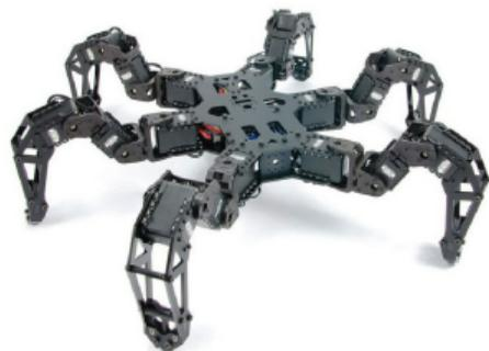
Hexapod with 3 servo motors (joints) per each leg has 18 servo motors in the total
