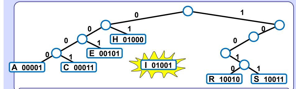
Inserting single key may result in creating more internal nodes. Insert I [01001].
