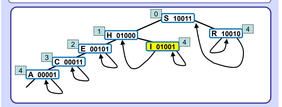
To insert N = 01110, we add a new node in between H and I to check bit 2, since that bit distinguishes N from H and I.
