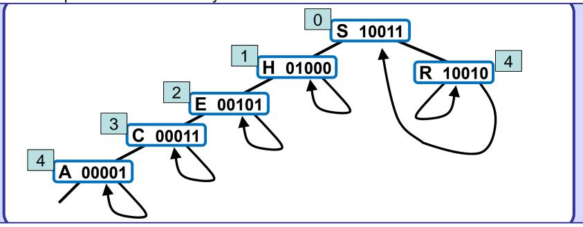
In an unsuccessful search for I = 01001, we move left at the root (since bit 0 of the key is 0), then take the right (up) link (since bit 1 is 1) and find that H (the only key in the trie that begins with 01) is not equal to I.
