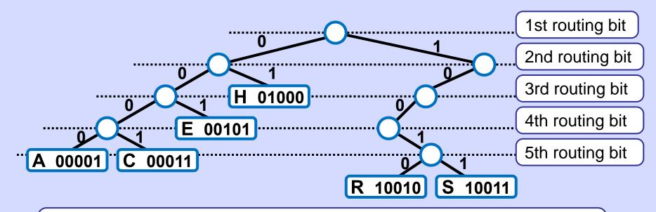
Tree height ≤ no. of routing bits = length of bit representation of keys
