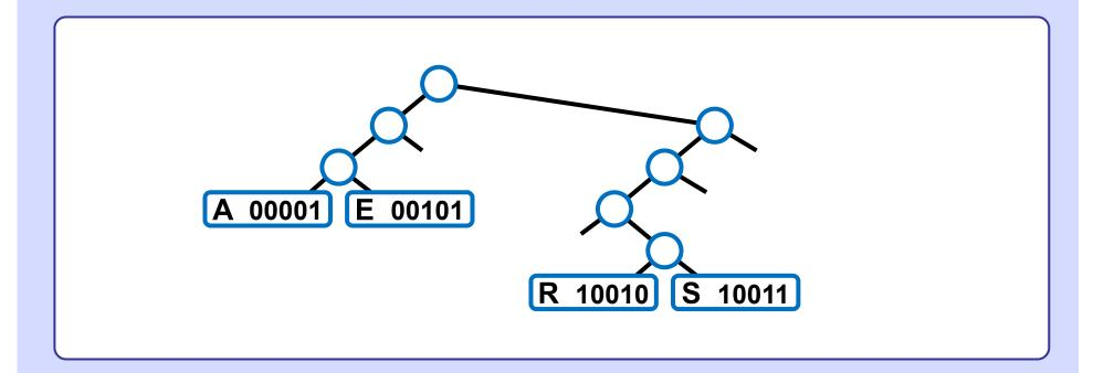
Null pointers in internal nodes are called null links. When trie has no null link it is a complete perfectly balanced binary tree containing 2<sup>d+1</sup>–1 nodes and 2<sup>d</sup> leaves.
