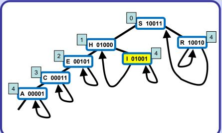
To insert I into the sample patricia trie, we add a new node to check bit 4, since H = 01000 and I = 01001 differ in only that bit (top). On a subsequent search in the trie that comes to the new node, we want to check H (left link) if bit 4 of the search key is 0; if the bit is 1 (right link), the key to check is I.
