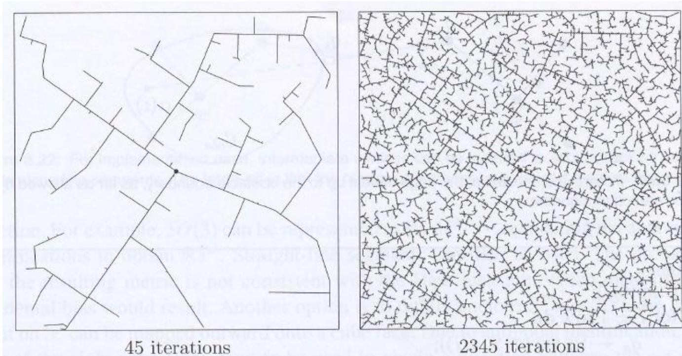
**Behavior of a RDT:** The initial iterations are very efficient/fast in approaching yet not visited areas. Subsequently, the coverage is refined – in a limit case, the method assures full coverage with probability =1
