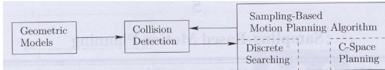
Sampling-based approaches use the collision avoidance as a „black-box“ which separates the planning mechanism from the geometric and kinematic model of the case. The gathered/derived samples from the world model serve to accomplish a discrete planning (decision-making process).
