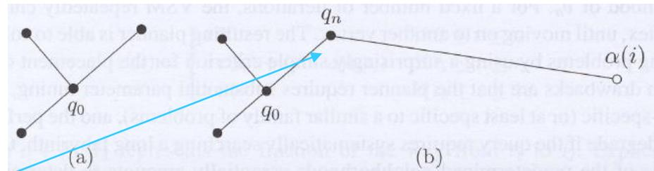
Function *NEAREST* determines a vertex of the so far existing tree  $S(\mathcal{G})$  which is closest to the newly generated vertex  $\alpha(i)$ ; there appears either 1 such a new object with creation of an edge, or 2 new edges (an edge is the closest  $\rightarrow$  splitting of the existing edge).
