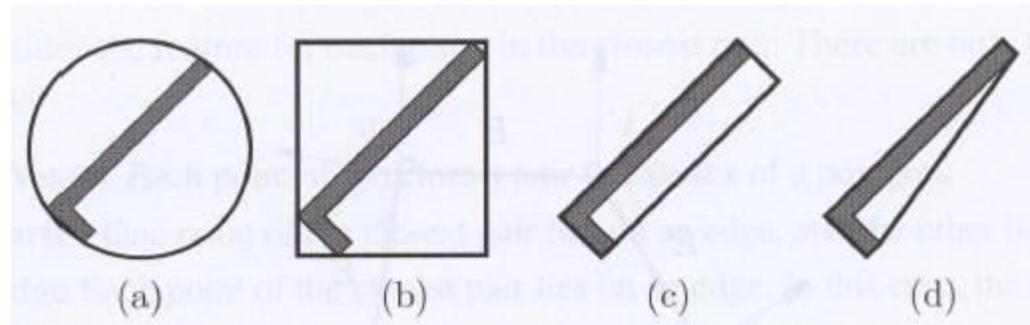
Various kinds of limiting regions (hulls): (a) circular sphere, (b) limiting rectangle; co-linear with the coordinate system, (c) oriented rectagle, (d) konvex hull
