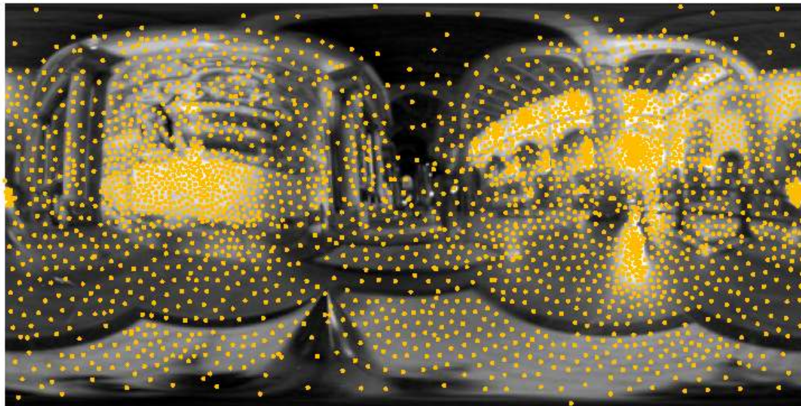
Figure 1: A high dynamic range 1024 \times 512 environment map [Debevec 98] sampled with 3000 point lights. In this image, importance density is represented by the lightness of the background. It took 0.064 seconds on a 2.6 GHz P4 to generate this point set. Similar results using a hardware accelerated Lloyd relaxation [Hoff et al. 1999] required 1 second, while Structured Importance Sampling [Agarwal et al. 2003] took 1393 seconds.
