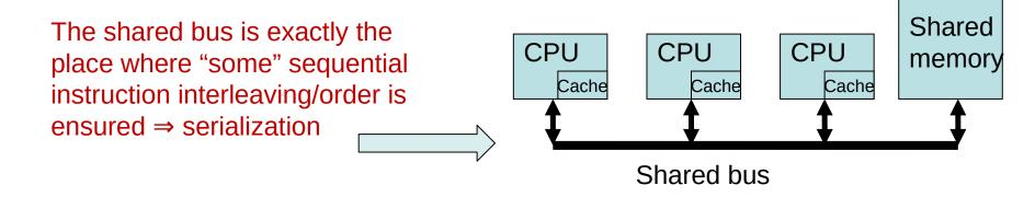
If processors (program) fulfill the sequential consistency conditions and the parallel system uses a shared bus, then the model of sequential consistency is achieved. Bus arbitration (acquire of time slot) in processor decides the memory operations order – the order can be perturbed for each collision occurrence, but the consistency conditions are preserved.
