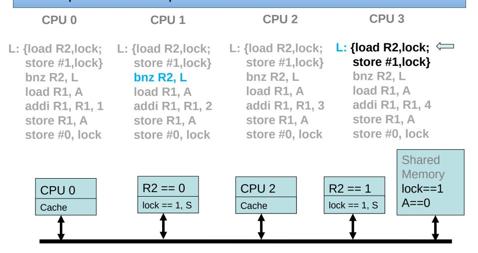
• CPU 3 obtains the bus. It requests to read "lock" value to R2. Snooping CPU 1 recognizes MemRead request and propagates the modified data to CPU 3 and memory. The corresponding line changes to S. CPU 3 receives the data and its final cache state is S as well.
