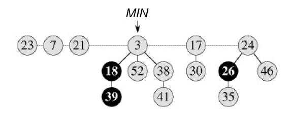
2. The situation after the minimum node z is removed from the root list and its children are added to the root list.
