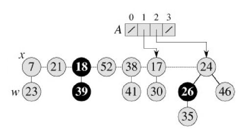
7. The node with key 17 has been linked to the node with key 7, which is still pointed to by *x*.
