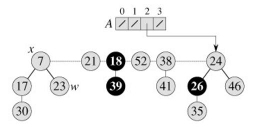
8. The node with key 24 has been linked to the node with key 7. Since no node was previously pointed to by A[3], at the end of the for each loop iteration, A[3] is set to point to the root of the resulting tree.
