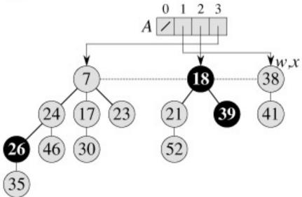
13. The Fibonacci heap after reconstruction of the root list from the array A and determination of the new MIN pointer.
