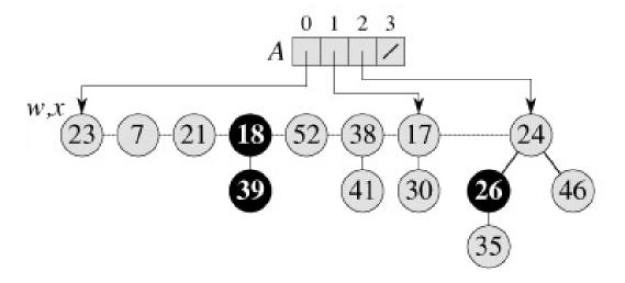
6. The Figure shows the situation after the first time through the *while* loop. The node with key 23 has been linked to the node with key 7, which is now pointed to by *x*.
