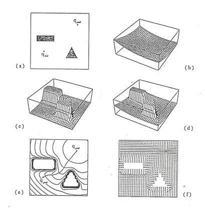
(a) The scene setup, (b) Attractive potential, (c) Repulsive potential, (d) Superposition of the repulsiveand attractive potentials, (e) Equivalent potentials lines, (f) Force vector field
