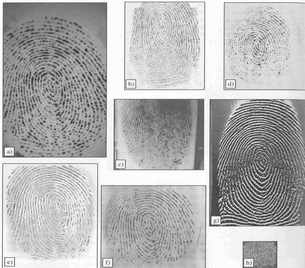
Figure 2.15. Fingerprint images of the same dry finger as acquired by different commercial scanners. Images are reported with right proportions: a) Biometrika FX2000, b) Digital Persona UareU2000, c) Identix DFR200, d) Ethenica TactilSense T-FPM, e) ST-Microelectronics TouchChip TCS1AD, f) Veridicom FPS110, g) Atmel FingerChip AT77C101B, h) Authentec AES4000.
