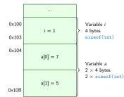
In this example, the variable allocation starts from the address  $0 \times 100$  just for visualization and better understandability. Automatic variables on the stack are usually allocated from the upper address to the lower ones.
