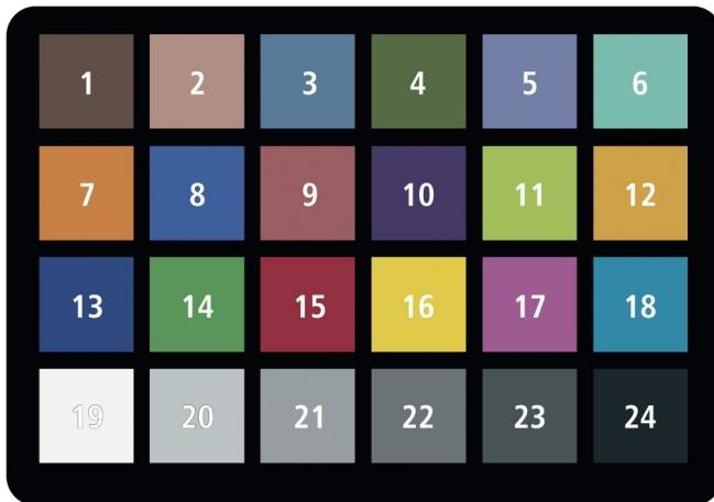
The data below is intended to be an average measurement of all ColorChecker Charts. ColorChecker Charts should be replaced every two years as fading of the colors will alter the values of the chart.
