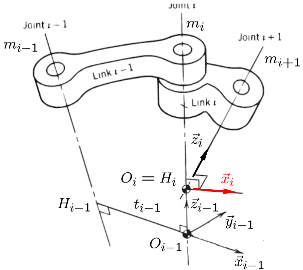
4.6 If  $m_i$  intersects  $m_{i+1}$ , then place  $\vec{x}_i$  in the direction perpendicular to  $m_i$ ,  $m_{i+1}$ , preferably to contain a sharp angle with  $\vec{x}_{i-1}$ .
