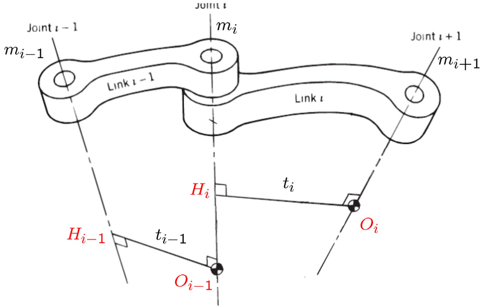
3.3 Find origins  $O_i = t_i \wedge m_{i+1}$  and points  $H_i = m_i \wedge t_i$ .
