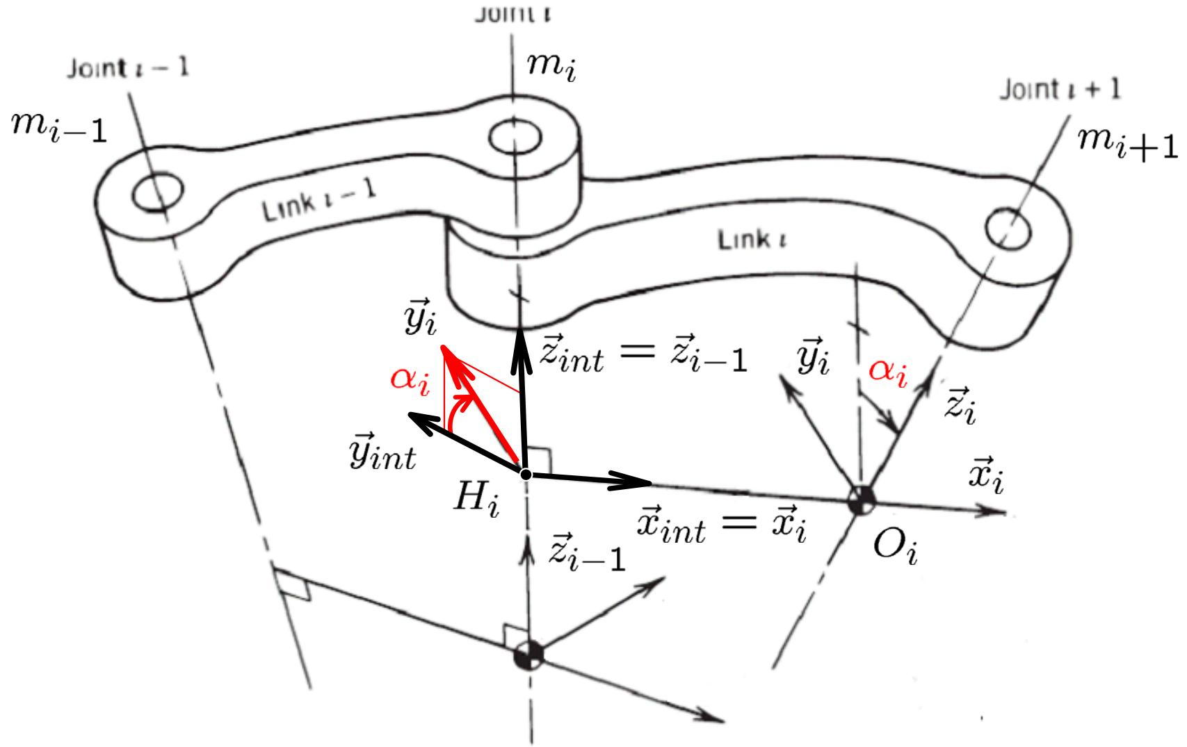
4.8 Construct the *intermediate coordinate system*
