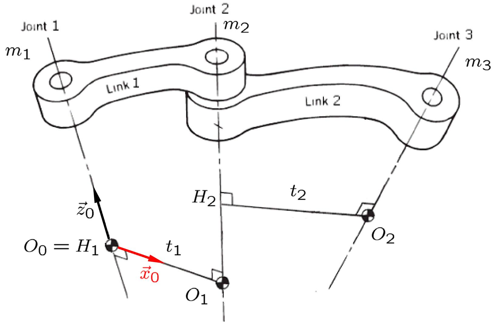
4.2 Choose axis  $\vec{x}_0$  along  $t_1$  in the direction from  $O_0$  to  $O_1$ . at will.
