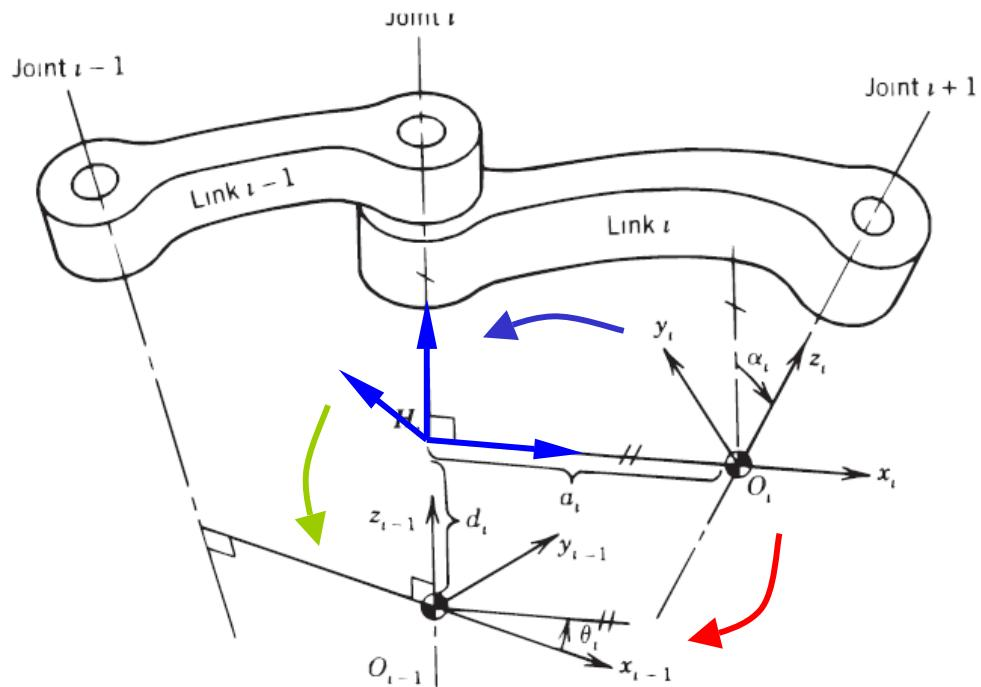
Transformation in a joint is described by 4 parameters
