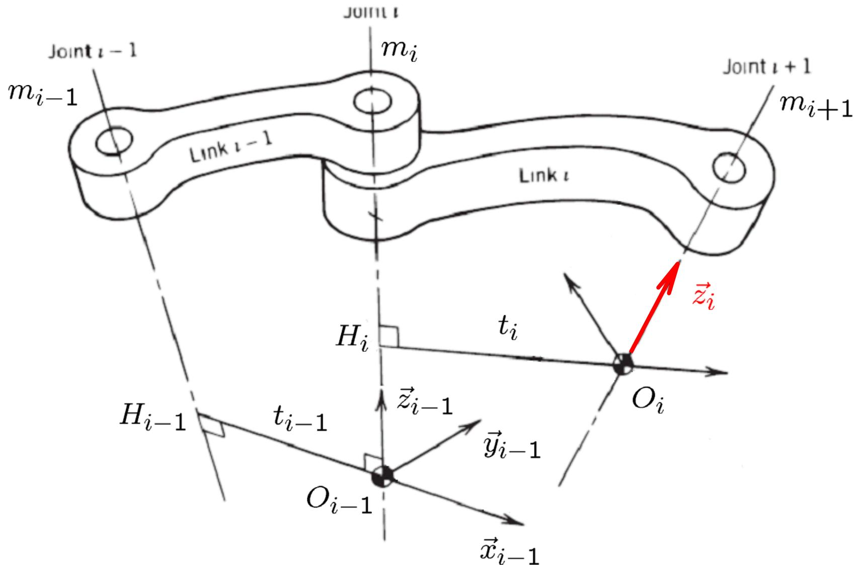
4.4 Place  $\vec{z}_i$  axis along the  $m_{i+1}$  axis, preferably to contain a sharp angle with the  $\vec{z}_{i-1}$ .
