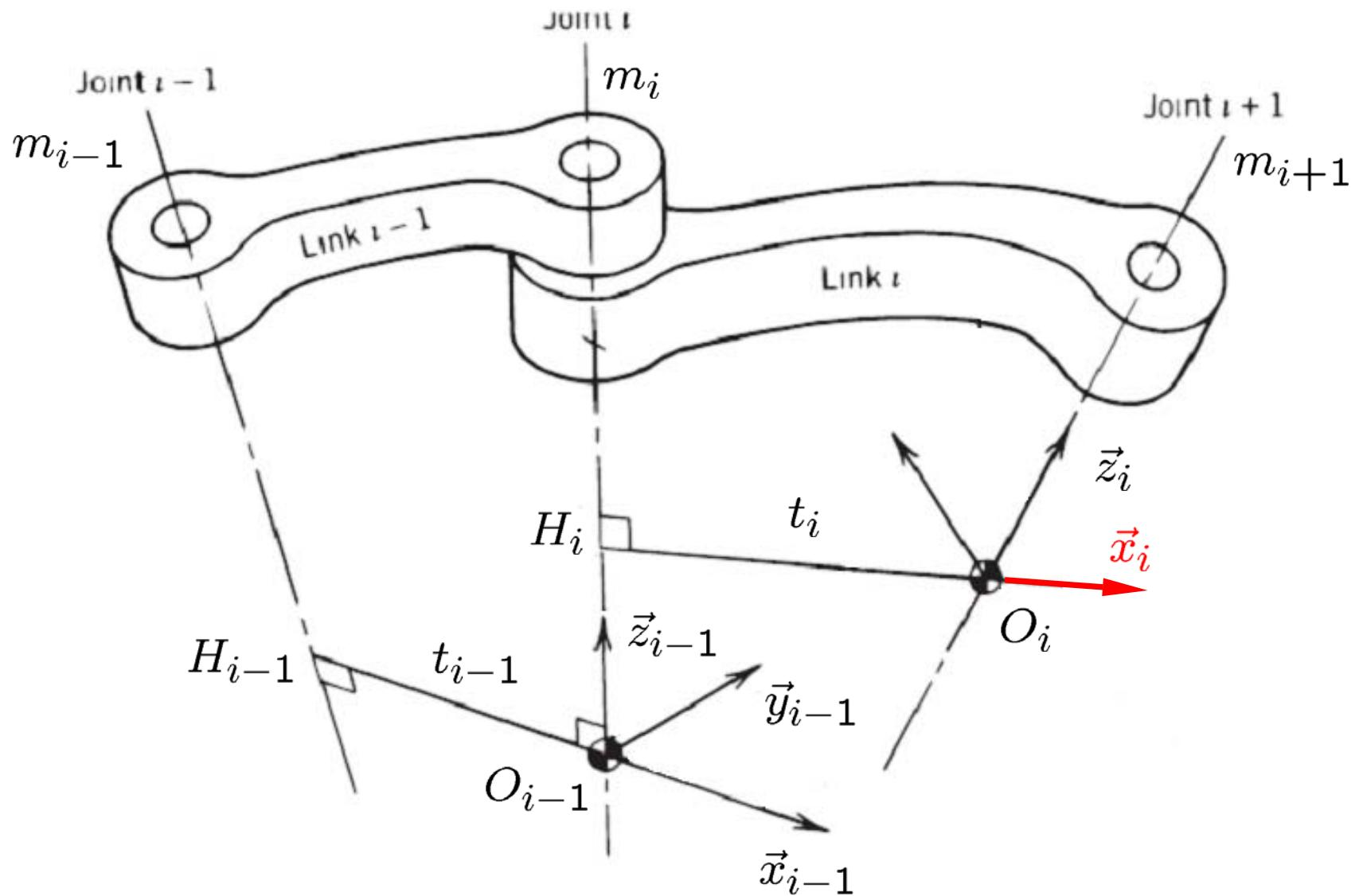
4.5 Place  $\vec{x}_i$  axis along  $t_i$  in the direction from  $H_i$  to  $O_i$ .
