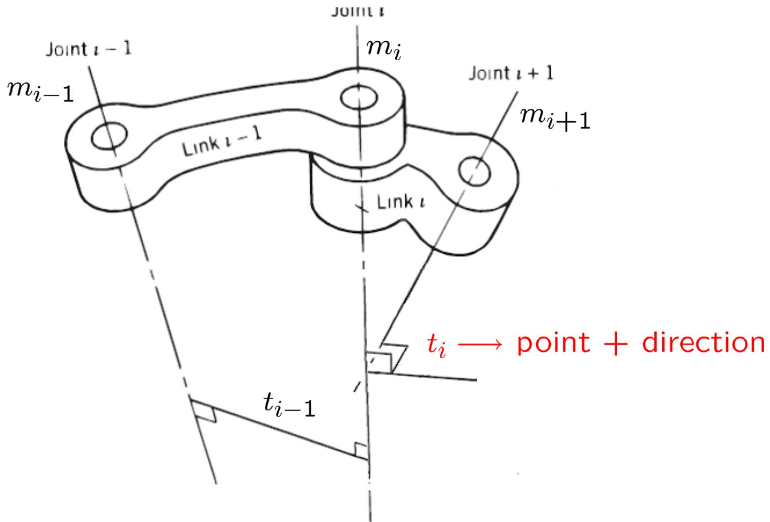
2.3 If  $m_i$  intersects  $m_{i+1}$ , the  $t_i$  becomes the intersection point and the direction perpendicular to  $m_i$ ,  $m_{i+1}$ .
