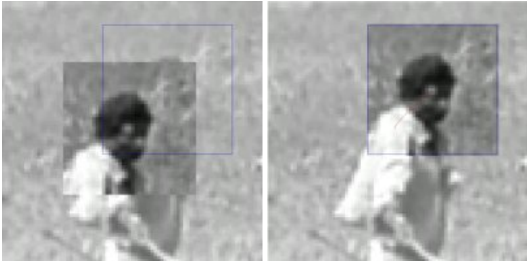
Figure 1.1: Goal is to align a template image T(\mathbf{x}) to an input image I(\mathbf{x}) , where \mathbf{x} is a column vector containing image coordinates [x, y]^\top . The I(\mathbf{x}) could be also a small sub-window within an image.
