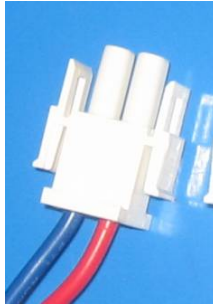
Figure 21. 2 pins connector used to connect the battery to the platform
