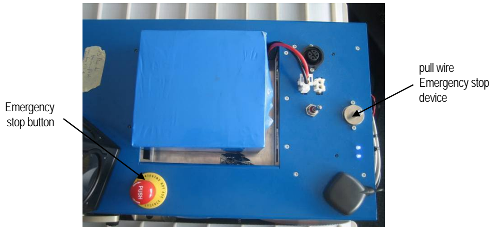
Figure 12. Emergency stop button and pull wire Emergency stop device
