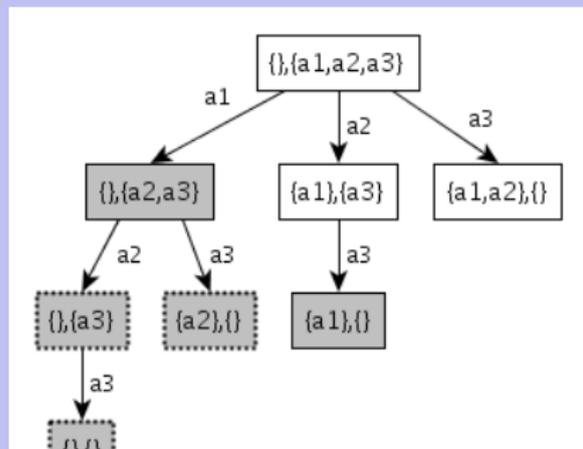
In gray states, the concept *Person* is satisfiable ( $R(Pe, D \cup P) = true$ ). States with a dotted border are pruned by the algorithm.
