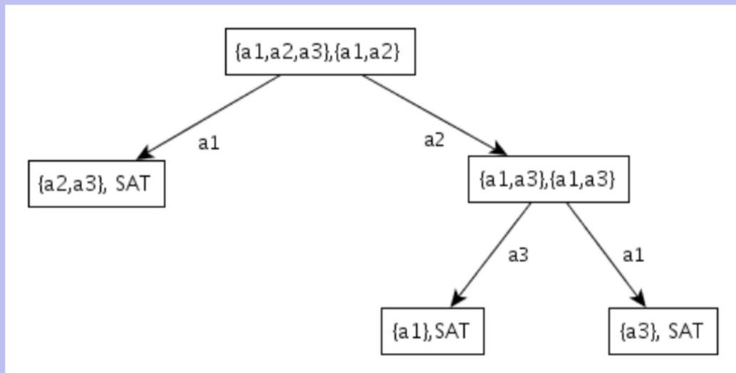
The algorithm ends up with two MUPSeS  $\{\alpha_1, \alpha_2\}$  a  $\{\alpha_1, \alpha_3\}$ . “For free” we got diagnoses  $\{\alpha_1\}$  a  $\{\alpha_2, \alpha_3\}$ .
