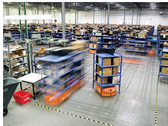
Kiva Systems (Amazon warehouse)
