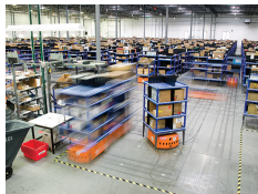
Kiva Systems (Amazon warehouse)
