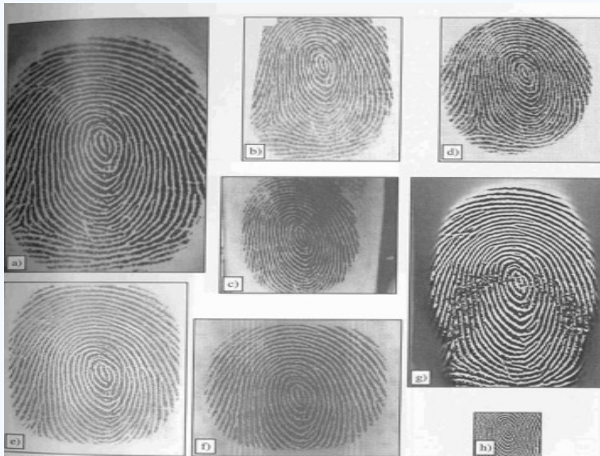
Figure 2.14. Fingerprint images of the same finger with ideal skin condition as acquired by different commercial scanners. Images are reported with right proportions: a) Biometrika FX2000, b) Digital Persona UareU2000, c) Identix DFR200, d) Ethentica TactiSense T-FPM, e) ST-microelectronics TouchChip TCS1AD, f) Veridicom FPS110, g) Atmel FingerChip AT77C101B, h) Authentec AES4000.
