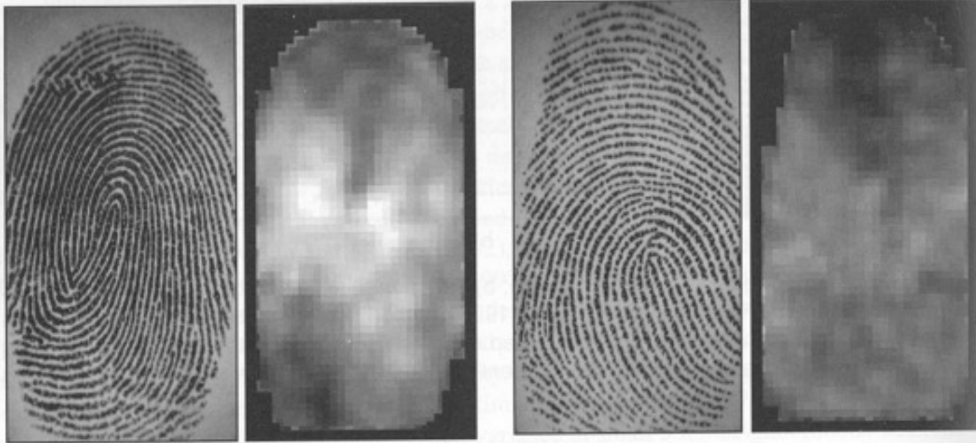
Figure 3.10. Two fingerprint images and the corresponding frequency image computed with the method proposed by Maio and Maltoni (1998a). A local 3 \times 3 averaging is performed after frequency estimation to reduce noise. Light blocks denote higher frequencies. It is quite evident that significant changes may characterize different fingerprint regions and different average frequencies may result from different fingers.
