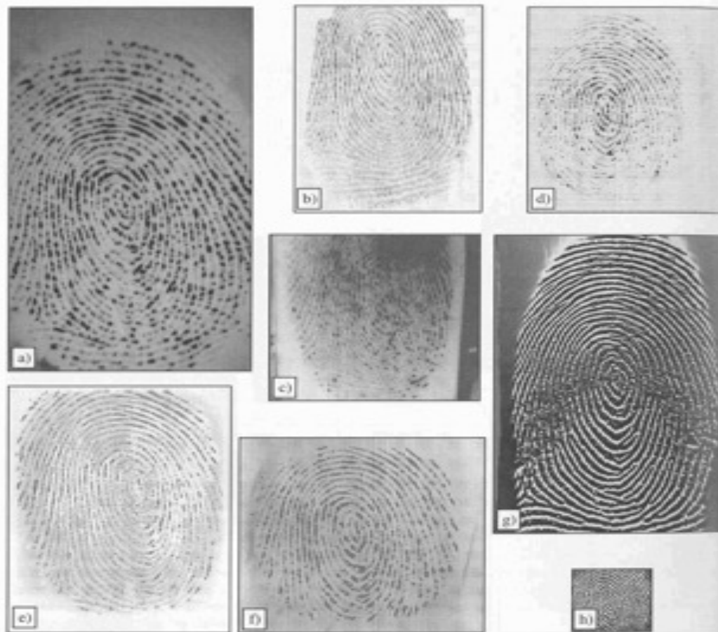
Figure 2.15. Fingerprint images of the same dry finger as acquired by different commercial scanners. Images are reported with right proportions: a) Biometrika FX2000, b) Digital Persona UareU2000, c) Identix DFR200, d) Ethentica TactiSense T-FPM, e) ST-Microelectronics TouchChip TCS1AD, f) Veridicom FPS110, g) Atmel FingerChip AT77C101B, h) Authentec AES4000.
