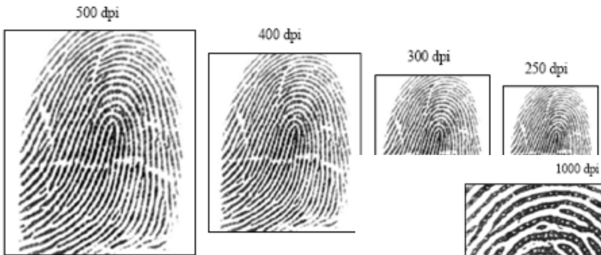
Figure 2.15. The fingerprint on the left, acquired at 50 lower resolutions: 400, 300, and 250 dpi, respectively.
