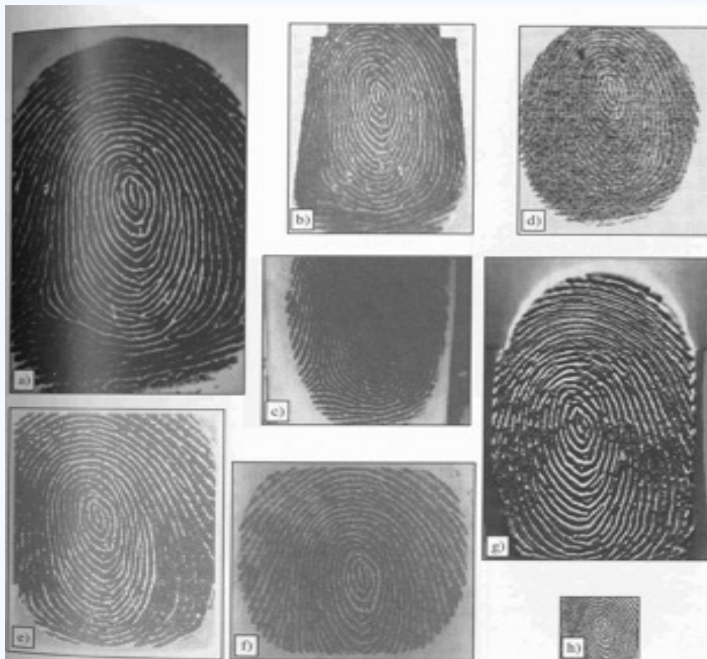
Figure 2.16. Fingerprint images of the same wet finger as acquired by different commercial scanners. Images are reported with right proportions: a) Biometrika FX2000, b) Digital Persona UareU2000, c) Identix DFR200, d) Ethentica TactiSense T-FPM, e) ST-Microelectronics TouchChip TCS1AD, f) Veridicom FPS110, g) Atmel FingerChip AT77C101B, h) Authentec AES4000.
