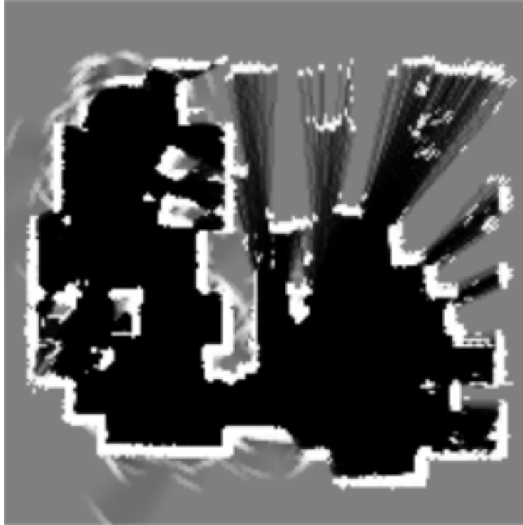
Fig.1.: An example of an occupancy grid. The lighter the cell the higher probability that it is occupied by an obstacle.
