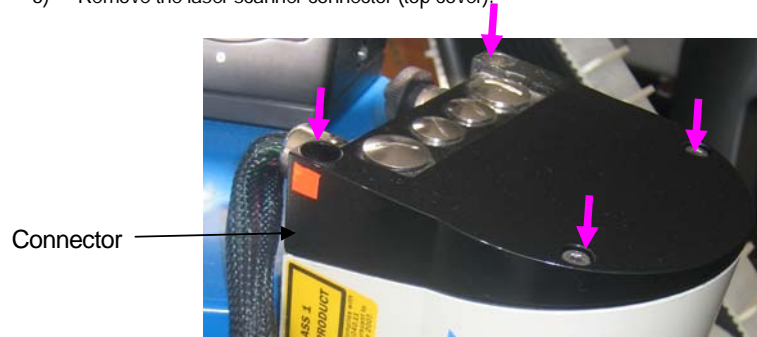
Figure 3. Remove laser scanner connector
