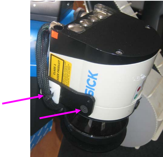
Figure 2. Unscrew the laser scanner
