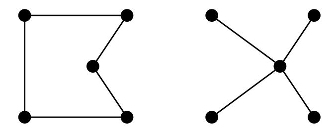
Minimum spanning tree can be computed in  $O(n^2)$  and is a lower bound on the shortest (open) tour
