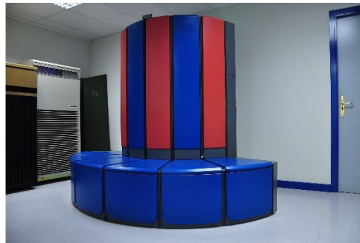
Cray X-MP (1982) parallel vector CPU
