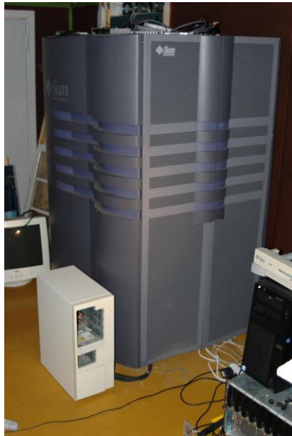
Sun Starfire 10000 (1997) 64 UltraSPARC CPUs
