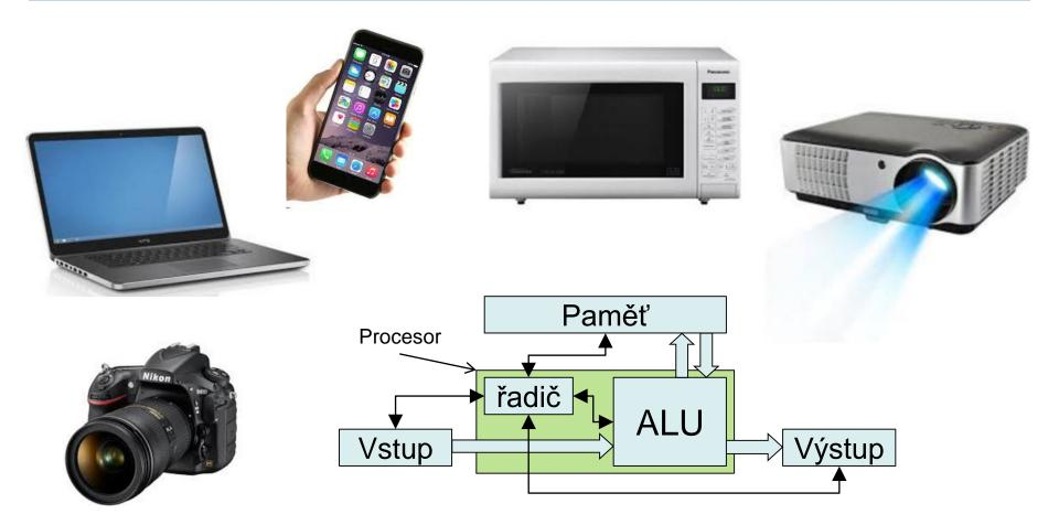
• The processor performs stored memory (ROM, RAM) instructions to operate peripherals, to respond to external events and to process data.
