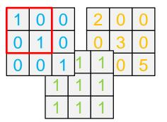
• replace elements in the first two rows and columns of the first sheet of the array (i.e. the matrix [1 0; 0 1]) with NaN elements
