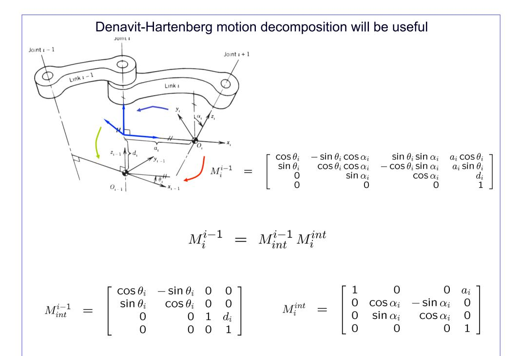
Given the position of the flange, i.e. the matrix Mand parameters of the mechanism, e.g.  $\alpha_i$ ,  $a_i$ ,  $d_i$ compute the control variables  $\theta_1$ ,  $\theta_2$ ,  $\theta_3$ ,  $\theta_4$ ,  $\theta_5$ ,  $\theta_6$
