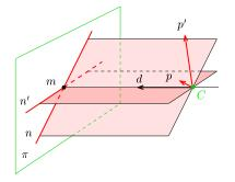
optical plane normal given by n  $\mathbf{p} = \mathbf{Q}^\top \mathbf{\underline{n}}$ optical plane normal given by n'  $\mathbf{p}' = \mathbf{Q}^\top \mathbf{\underline{n}}'$
