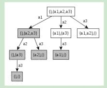
In gray states the following holds:  $R(C, D \cup P) = true$ . States with a dotted border are pruned by the algorithm.
