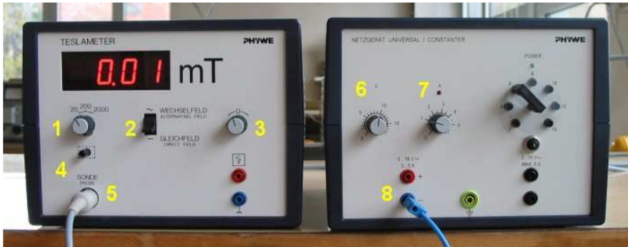
Figure 2. Teslameter and power supply unit.
