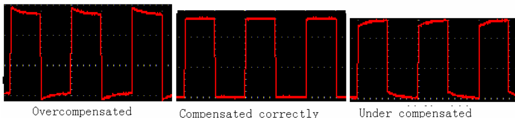
Fig. 4-5 Displayed Wave Forms of the Probe Compensation
