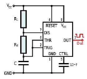
In astable mode, the 555 timer puts out a continuous stream of rectangular pulses having a specified frequency. Resistor  $R_1$  is connected between  $V_{CC}$  and the discharge pin (pin 7) and another resistor ( $R_2$ ) is connected between the discharge pin (pin 7), and the trigger (pin 2) and threshold (pin 6) pins that share a common node. Hence the capacitor is charged through  $R_1$  and  $R_2$ , and discharged only through  $R_2$ , since pin 7 has
