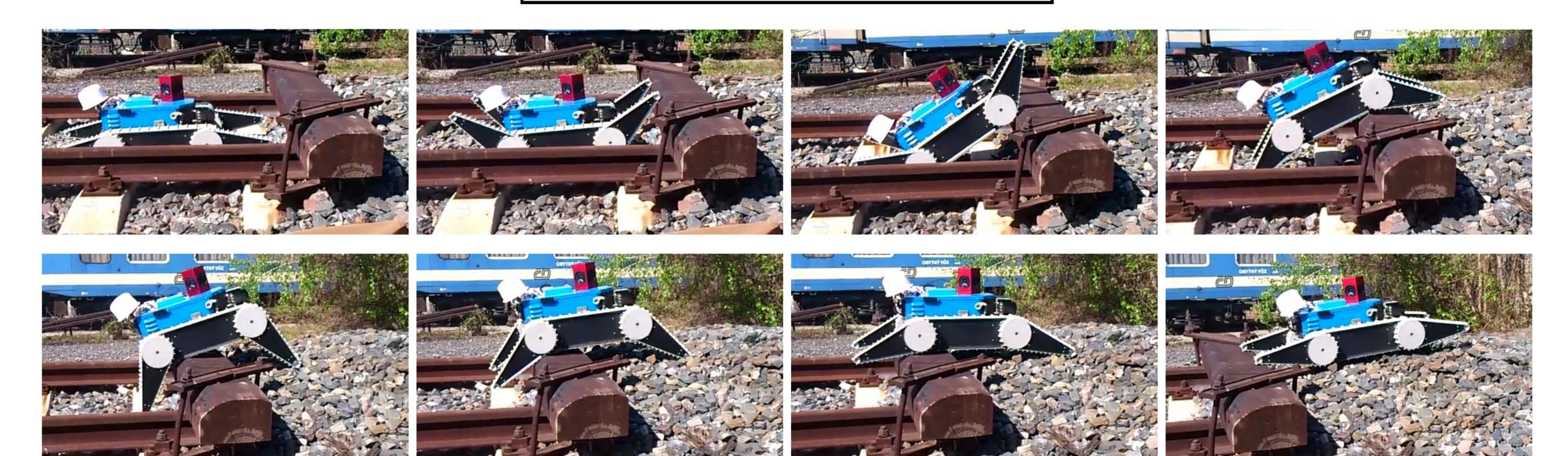
Only the forward speed is controlled manually. Flippers bend automatically.
