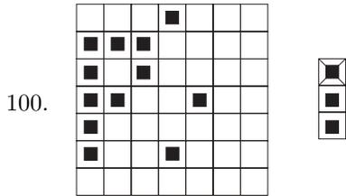
A binary mathematical morphology example. The left image gives the point set  $A$ ; the right image gives the structuring element  $B$ . Its representative pixel is denoted by a cross. Draw the result of the erosion  $A \ominus B$ .
