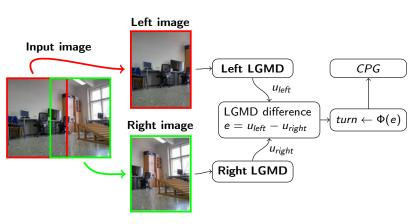
A mapping function: Φ from the output of the LGMD vision system to the turn parameter of the CPG
