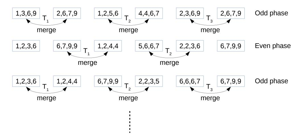
Use barrier to synchronize threads between phases
