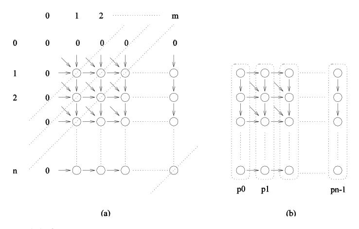
(a) Computing entries of table for the longest-commonsubsequence problem. **Computation proceeds along the dotted diagonal lines**. (b) **Mapping elements** of the table to processing elements.
