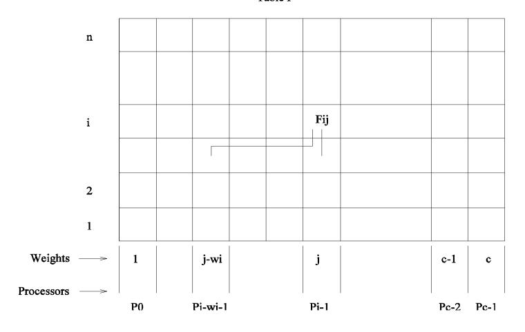
Computing **entries of table** *F* for the 0/1 knapsack problem. The computation of entry *F*[*i*,*j*] requires communication with processing elements containing entries *F*[*i*-1,*j*] and *F*[*i*-1,*j*-w<sub>i</sub>]<sup>2</sup>.
