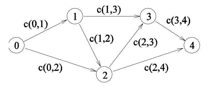
A graph for which the shortest path between nodes 0 and 4 is to be computed.
