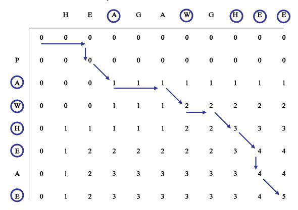
The F table for computing the LCS of the sequences. The LCS is A W H E E.
