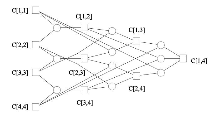
A nonserial polyadic DP formulation for finding an optimal matrix parenthesization for a **chain of four matrices**. A **square node represents the optimal cost** of multiplying a matrix chain. A **circle node represents a possible parenthesization**.
