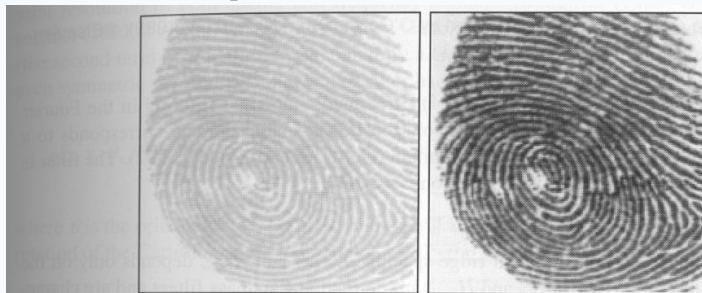
Figure 3.25. An example of normalization with the method described in Hong, Wan and Jain (1998) using ( m_0 = 100 , v_0 = 100 ). ©IEEE.
