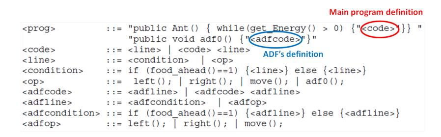
A header of a single ADF, adf0(), is defined so only a body of this particular ADF can be generated using the chromosome.
