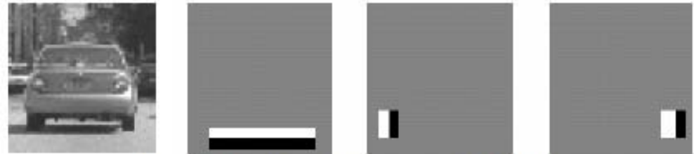
Figure 2 First three filters selected by Adaboost
