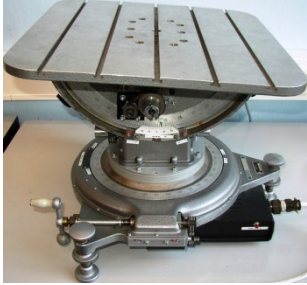
Fig. 4. Rotational Tilt Platform (ROTIP) for automatic positioning and precise attitude angle measurement; granted angular resolution below 2.6 arcsec [19, p. 243].
