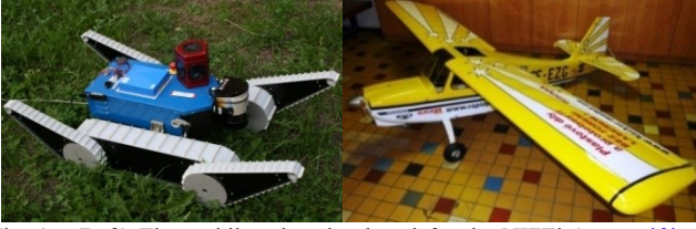
Fig. 1. (Left) The mobile robot developed for the NIFTi ( www.nifti.eu ) project; hardware design by Blue Botics ( www.bluebotics.com ), sensors equipped: Point Grey Ladybug 3 camera, rotating 2D laser scanner SICK LMS-151, Xsens MTi-G unit; (Right) The Bellanca Super Decathlon XXL aircraft model: 3m wing span, 13-15 kg weight, produced by Hacker Model Production Inc ( www.hacker-model.com ).
