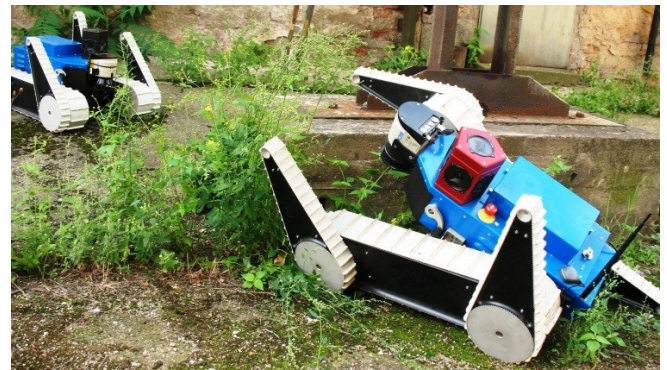
Figure 1. The mobile robot developed for the NIFTi ( www.nifti.eu ) project; hardware design by BlueBotics ( www.bluebotics.com ), sensors equipped: Point Grey Ladybug 3 camera, rotating 2D laser scanner SICK LMS-151, Xsens MTI-G unit
