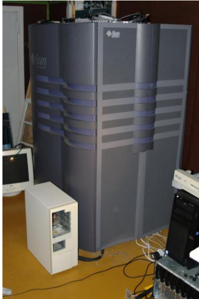
Sun Starfire 10000 (1997) 64 UltraSPARC CPUs
