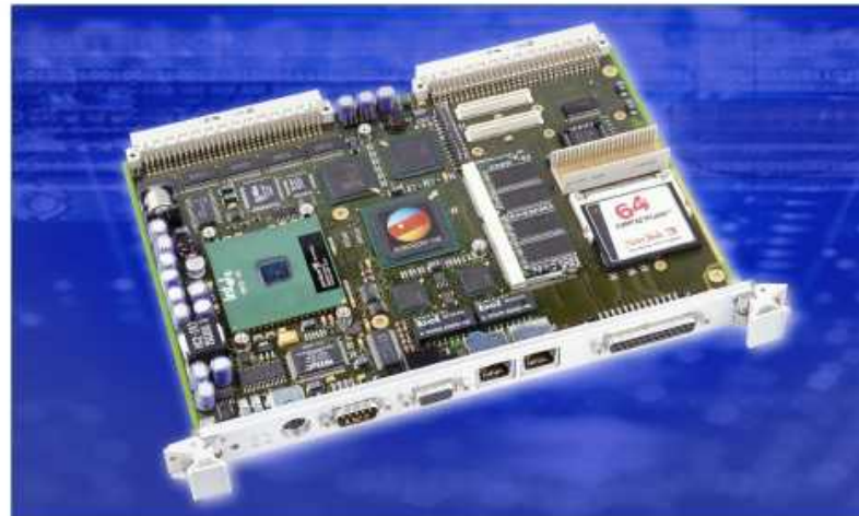
EUROCOM 148 VMEbus CPU board American ELTEC, Inc.
