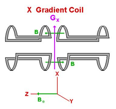
Fast on/of switching induces eddy currents  $\Rightarrow$  active shielding
