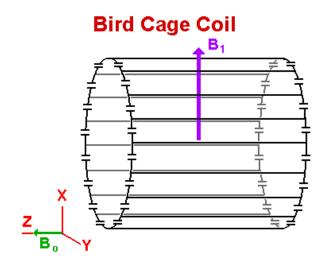
Consider a cylinder oriented along the z-axis with the current distribution  $I_z = I_0 \cos \phi$  in its jacket. This gives a homogeneous transversal field.
