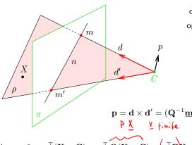
optical ray given by  $m extbf{d} = \mathbf{Q}^{-1}\mathbf{m}$ optical ray given by m'  $\mathbf{d}' = \mathbf{Q}^{-1}\mathbf{m}'$
