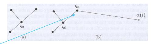
Function *NEAREST* determines a vertex of the so far existing tree S(G) which is closest to the newly generated vertex  $\alpha(i)$ ; there appears either 1 such a new object with creation of an each new vertex (the closest is a vertex), or 2 new edges (an edge is the closest  $\rightarrow$  splitting of the existing edge).
