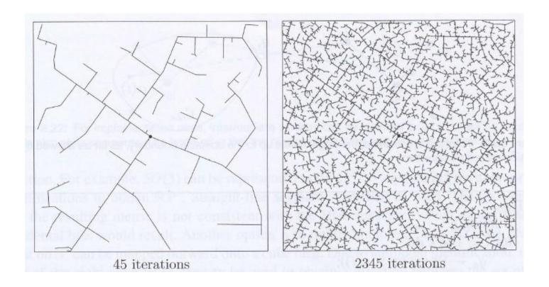
**Behavior of a RDT**: The initial iterations are very effcient/fast in approaching yet not visited areas. Subsequetly, the coverage is refined – in a limit case, the method assures full coverage with probability =1
