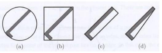
Various kinds of limiting regions (hulls): (a) circular sphere, (b) limiting rectangle; co-linear with the coordinate system, (c) oriented rectagle, (d) konvex hull
