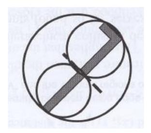
Circular sphere denotes the vertex that describes the whole object. After further splitting (dashed line), 2 smaller circles represent description of both the halves of the original object (2 vertices at lower level)
