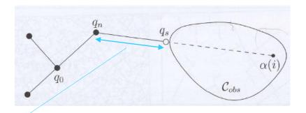
The least admissible distance of the point  $q_s$  from the border of the obstacle – this is denoted by the applied algoritm for collision avoidnace; in some cases with small distances of  $q_n$  from the obstacle the edge  $q_n q_s$  needs not to be created at all..
