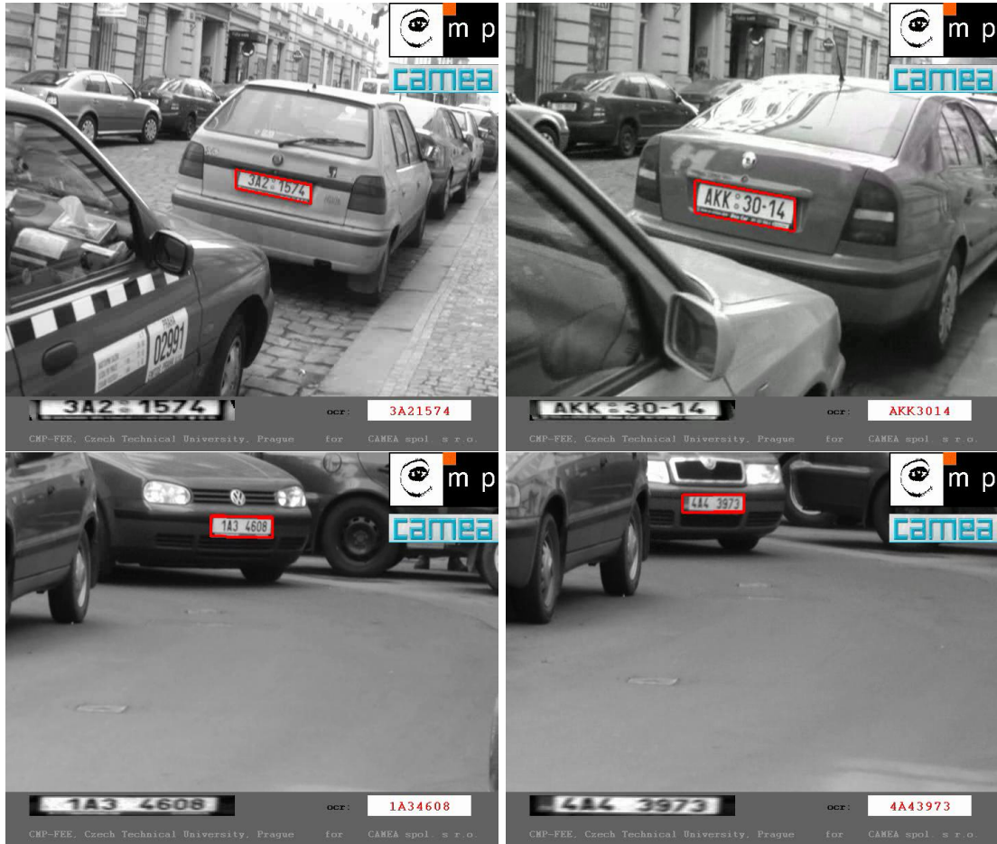
Figure 6: Example of a commercial application for registration plate recognition in a video. Demo videos can be found at http://cmp.felk.cvut.cz/cmp/courses/X33KUI/Videos/RP_recognition/ and you have also seen a demonstration of the first algorithm in the first seminar.
