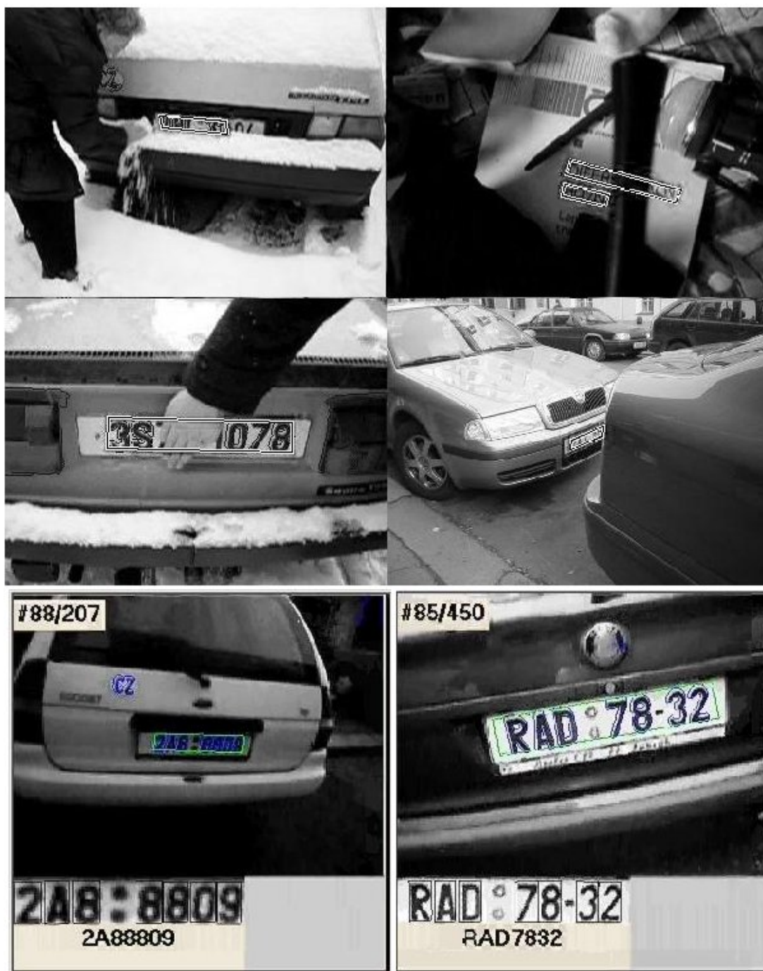
Figure 5: Example of an automatic text localization in an image. Further information can be found at http://cmp.felk.cvut.cz/~zimmerk/lpd/index.html
